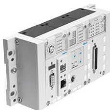
Figura 6.1 – PLC Festo CPX-CEC
